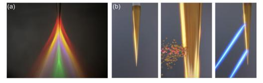
**Fig. 35** Tapered optical fibers as neuronal interfaces. (a) Example of how modes of different order outcouple at different sections of a TF. Image is in false colors. (b) High resolution patterning allows structuring the non-planar edge of metal-coated tapered optical fibers.
