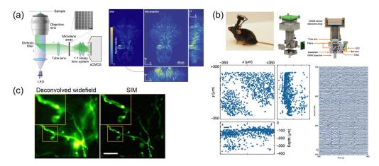
**Fig. 39** Computational microscopy enables novel imaging capabilities. (a) Light field microscopy enables single-shot high-speed volumetric neuronal imaging. (b) Miniaturized light field microscope allows volumetric neuronal recording in freely moving mice. (c) Structured illumination microscopy achieves super-resolution reconstruction of dendrites expressing ChR2-GFP on the mouse brain *in vivo*. (689)
