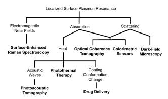
**Scheme 1** Localized surface plasmon resonance (LSPR) is the origin of a number of interesting phenomena observed with gold nanostructures. These properties have enabled a number of applications, which are indicated in bold.
