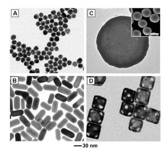
Fig. 2 Commonly studied gold nanostructures: (A) multiply twinned gold nanoparticles (often referred to as nanospheres), (B) gold nanoshells (silica beads coated with a polycrystalline gold layer), (C) gold nanorods, and (D) gold nanocages. The scale bar in the inset is 200 nm. Modified with permission from ref. 53 (A, B) and ref. 63 (C), copyright 2010 Wiley and 2007 American Chemical Society, respectively.
